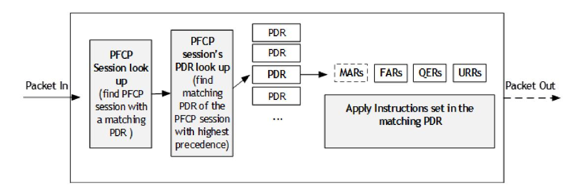
PDR – Packet Detection Rule FAR – Forwarding Action Rule QER – QoS Enforcement Rule URR – Usage Reporting Rule BAR – Buffering Action Rule MAR – Multi-Access Rule
