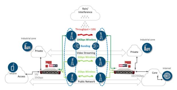
delay. This enables connecting multiple point-to-point wireless radio devices, with an option to include other transport interface types. This bonding technology ensures optimum performance and improves the transmitted throughput by dynamically distributing data along multiple wireless links of different speeds and technologies. This allows operators to increase the maximum transmission distance and overcome interruptions or slow wireless transmission due to inclement weather.
